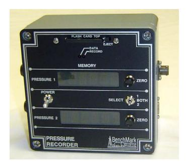
This system is designed to display wellhead pressure inside of a wireline unit. The system consists of the pressure display panel, pressure transducers, and cables.
